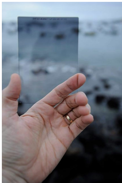
Holding the graduated neutral density filter up, you can see how the filter will darken the scene.
