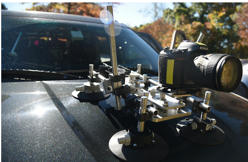
Nikon D750 & AF-S NIKKOR 24-120mm f/4G ED VR lens rigged up to capture driver POV footage for Ride Along.
