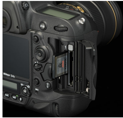
The Nikon D4 and D4S (shown here) DSLR cameras feature two media card slots—one XQD and one CompactFlash.
