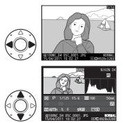
To end playback and return to shooting mode, press the shutter-release button halfway.
