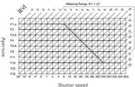
The maximum and minimum values for EV vary with sensitivity (ISO equivalency). Matrix metering reduces to  $17\frac{1}{3}$  any EV that exceeds  $17\frac{1}{3}$  at a sensitivity of ISO 200 equivalent.
