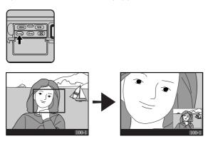
The center of the image will be enlarged to fill the monitor. To view other areas of the photograph, press the multi selector. To cancel zoom and return to normal playback, press the **FUNC** button.
