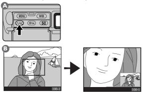
For approximately two seconds after you press the **FUNC** button to zoom in on the image, or after you press the multi selector to scroll the image, a thumbnail showing your current position in the image will appear in the bottom right corner of the display.
