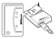
CHARGE lamp starts blinking when battery is inserted. Charging is complete when lamp stops blinking.
