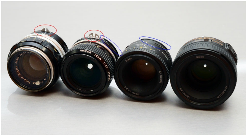
(l. to r.) Non-Ai lens with the meter coupling shoe circled in red; Ai lens with the meter coupling shoe circled in red and the meter coupling ridge circled in blue; AF-D lens with the meter coupling ridge circled in blue; and AF-S lens. Neither the Non-Ai lens nor the AF-S lens have a meter coupling ridge.
