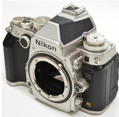
The Df camera is unique in that it can accept older non-Ai lenses as well as Ai lenses and current AF lenses (AF, AF-D, AF-S). Depending upon the lens you want to use, you'll adjust the lever (circled in red) up or down.
