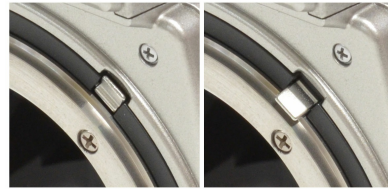
(l.) Meter coupling lever of the Nikon Df lowered (so it will engage the lens) and (r.) raised (out of the way). When attaching a Non-Ai lens to the camera, you must raise the meter coupling lever out of the way. When attaching an Ai lens, AF, AF-D or AF-S lens, the meter coupling lever needs to be lowered so it can engage the lens.
