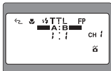
Display in dual-light close-up flash operation (in TTL mode)
