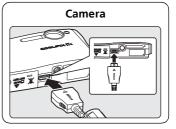
Make sure that the plugs are in the correct orientation. Inserting the plugs incorrectly may damage the COOL-STATION.
