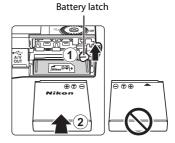
Inserting the Battery Correctly
