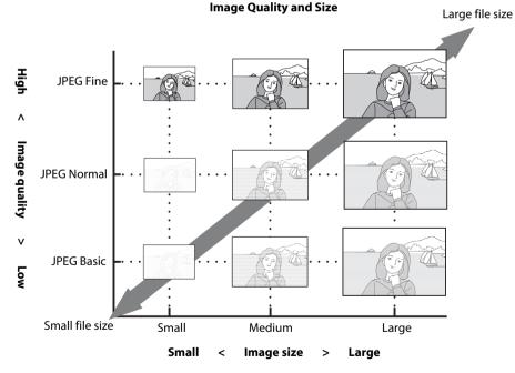
The approximate maximum file size of individual photographs and the total number of photographs that can be recorded at the selected setting are also shown in the Quick settings display while image quality or size options are displayed. Use the display only as a guide. Typical file sizes are listed in "Memory Card Capacity and Image Quality/Size" (**W** 178).
