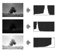
Increasing exposure compensation shifts tone distribution to the right. Tone distribution shifts to the left when exposure compensation is decreased. If bright ambient lighting makes it difficult to see the display in the monitor, the histogram can be used to get an idea of overall exposure.
