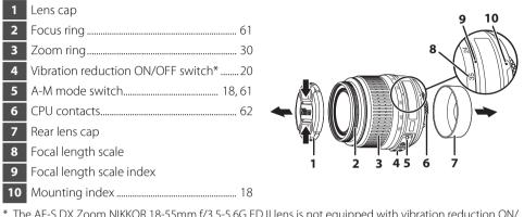
The AF-S DX Zoom NIKKOR 18-55mm f/3.5-5.6G ED II lens is not equipped with vibration reduction ON/ OFF switch.
