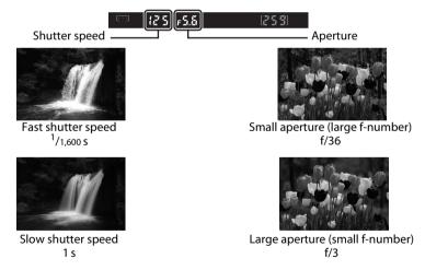
If the ISO sensitivity setting is changed (🔀 53, 111), the range of shutter speed and aperture settings that will achieve optimal exposure also changes.
