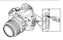
When the camera establishes communication with the GP-1, a size icon will appear in the information display. Photo information for pictures taken while the size icon is displayed will include an additional page of GPS data (\$\sup\$121). GPS data are only recorded when the size icon is displayed; confirm that the icon appears in the
