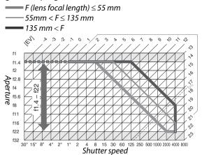
The maximum and minimum values for EV vary with ISO sensitivity; the above graph assumes an ISO sensitivity of ISO 200 equivalent. When matrix metering is used, values over  $17^{1/3}$  EV are reduced to  $17^{1/3}$  EV.
