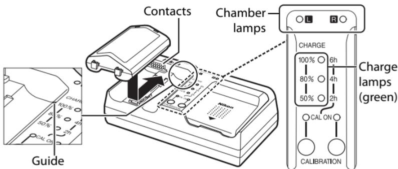
Insert the battery (terminals first), aligning the end of the battery with the guide and then sliding the battery in the direction indicated until it clicks into place. The chamber lamp and charge lamps will flash slowly while the battery charges:
