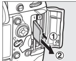
**CompactFlash memory cards:** Press the eject button (①) to partially eject the card (②). The memory card can then be removed by hand. Do not push on the memory card while pressing the eject button. Failure to observe this precaution could damage the camera or memory card.
