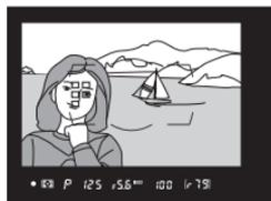
AF-area mode can be selected by pressing the AF-mode button and rotating the sub-command dial until the desired setting is displayed in the viewfinder and top control panel.
