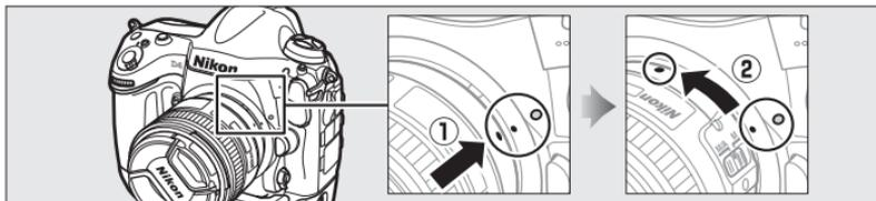
Keeping the mounting index on the lens aligned with the mounting index on the camera body, position the lens in the camera's bayonet mount (1). Being careful not to press the lens-release button, rotate the lens counter-clockwise until it clicks into place (2).
