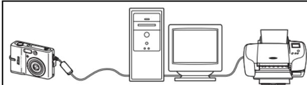
Use the supplied PictureProject software to copy pictures to a computer, and then organize, browse, edit, and save those pictures. Connect the camera to the computer using the supplied USB cable. You can also print pictures from a printer connected to the computer using PictureProject installed in the computer.
