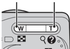
When the camera is zoomed in to the maximum magnification (3×), holding **T** (🔍) down triggers digital zoom. The subject is magnified up to 4×, for a total magnification of 12×.
