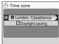
When daylight saving time ends, turn [Daylight saving] off from the [Date] menu (90) in the setup menu (87). The camera's clock is automatically set back one hour.
