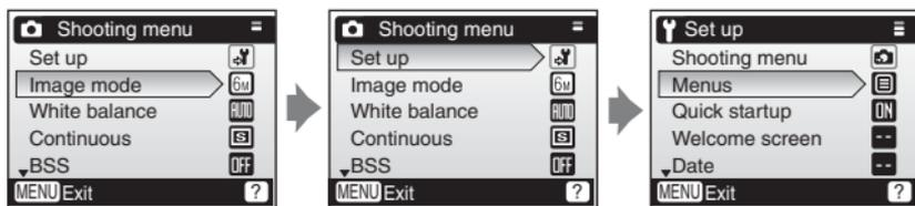
Display the menu screen Press the multi selector **▲** or **▼** to select [Set up] and press **OK**.
