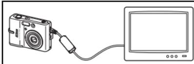
View pictures on a TV by connecting the camera via the Audio/Video Cable EG-CP14, supplied with the L11 or available separately for the L10.
