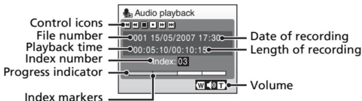
Volume can be adjusted with **W** (⏮)/**T** (⏭) during playback. Playback controls are displayed at the top of the monitor. Press ◀ or ▶ to choose a control, then press **OK** to perform the selected operation.
