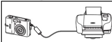
Connect your camera directly to a Pict-Bridge-compatible printer. Use the supplied USB cable to connect the camera to a printer for direct printing.
