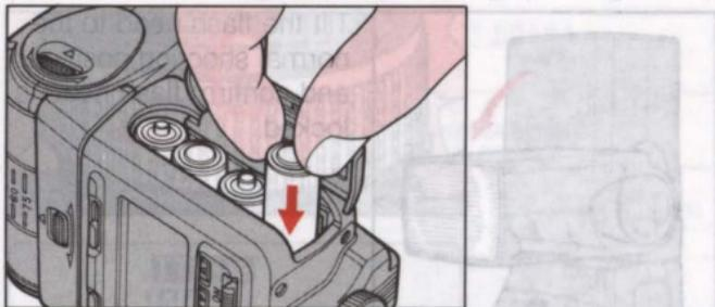
Use either 1.5V AA-type penlight alkaline-manganese or 1.2V NiCd batteries.
