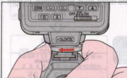
Turn locking wheel to tighten.
