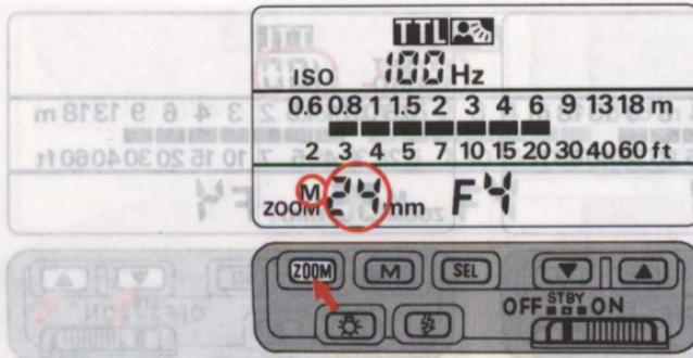
It is also possible to select your desired angle of coverage manually, by pressing the zoom button [ZOOM]. In the LCD panel, "M" appears above "ZOOM" indicator.
