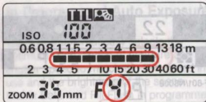
Confirm the shooting distance range in the SB-24's LCD panel. The shooting distance range is automatically indicated by the distance indicator bars.
