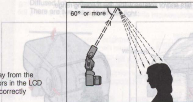
1. Select a ceiling or wall to bounce the flash from. In color photography, only use bounce with white surfaces. Otherwise, color photographs will come out with an unnatural color cast similar to that of the reflecting surface.
