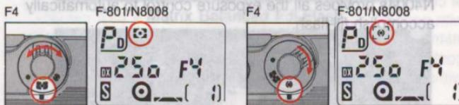
To select either Matrix Metering or Center-Weighted Metering, use the F-801/N8008's metering system selection button, or for the F4, selection dial.
