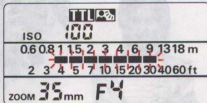
If shooting distance is within 1.5m (approx. 5ft.), tilt the flash head down to the -7° position so the flash light covers the subject. In this case, the shooting distance indicators in the LCD panel blink.
