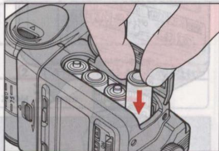
3. Load four 1.5V AA-type penlight alkaline-manganese or 1.2V NiCd batteries into the battery chamber. Be sure to follow the
