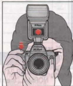
When ambient light is insufficient for autofocus operation, the AF illuminator automatically turns on to start operation. If ambient light is sufficient, the AF illuminator does not light up.
