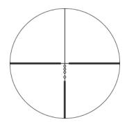
This simple, effective reticle design can be custom tailored for the trajectory of your ammunition. The accuracy circles on the lower vertical crosshair enable you to accurately compensate for bullet drop out to at least five hundred yards with most calibers. Nikon has designed this BDC reticle to blend simplicity with accuracy – a difficult challenge considering the huge number of variables involved in placing a bullet drop compensating scope on a rifle. These would include:
